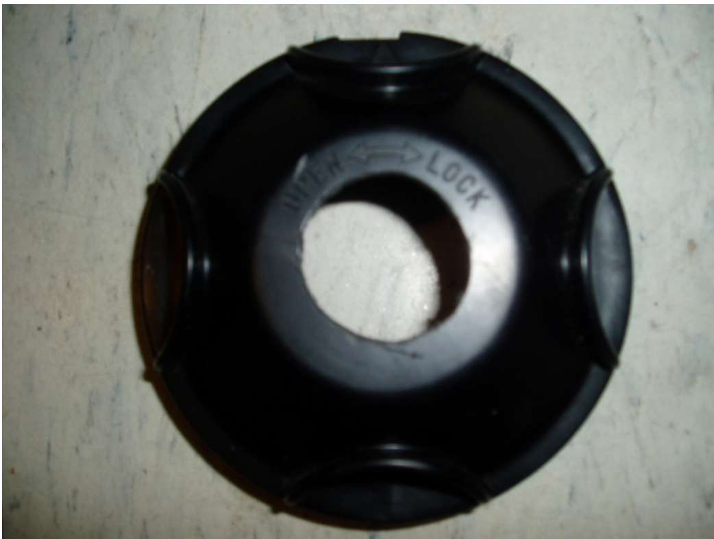
Use a dremil and make a round hole in the middle of the headlight dust cover for the rubber grommet.
