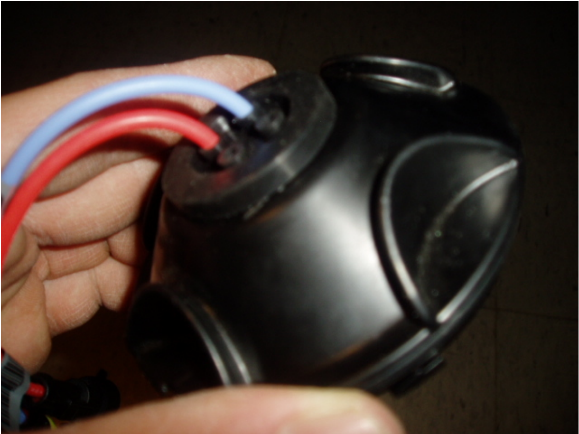
If installed properly, this is how the grommet should cover the hole that you made in the dust cover.
